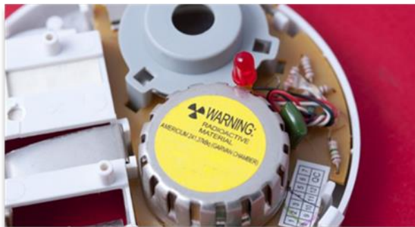
Figure 6. Am-241 radioactive isotope in an ionisation smoke detector (HomeHow 2021)
