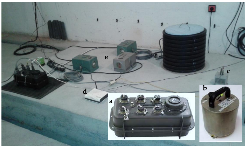
Figure 1. Seismological equipment of a standard monitoring seismic station consisting of (a) data logger, (b) three-component seismometer located in the black heat-insulating cover, (c) accelerometer and d) network communication module. There are also a museum exhibit of SM-2M short-period, single-component seismometer (e).
